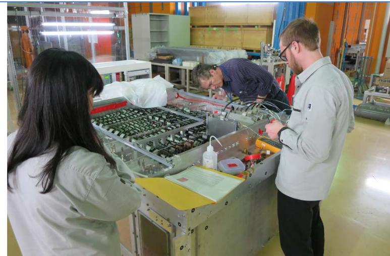
Gluing spacer one by one.
